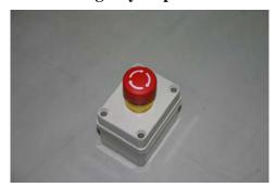
It is fitted at the unit and makes stop of all crane function in emergency. To restore function, turn to the switch to the clockwise.
